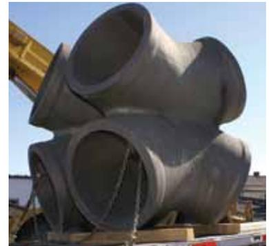
Figure 9: One of the nodes ready to ship to the machine shop. Courtesy of Bradken Inc.
