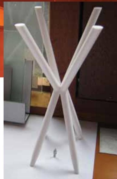
Figure 5: Rapid prototype of a full delta frame at 1:100 scale. Courtesy of Sweeny Sterling Finlayson & Co Architects Inc. and Allied Properties REIT.
