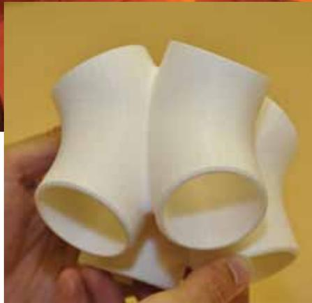
Figure 4: Rapid prototype of the cast steel node at 1:20 scale. Courtesy of Cast ConneX Corporation.
